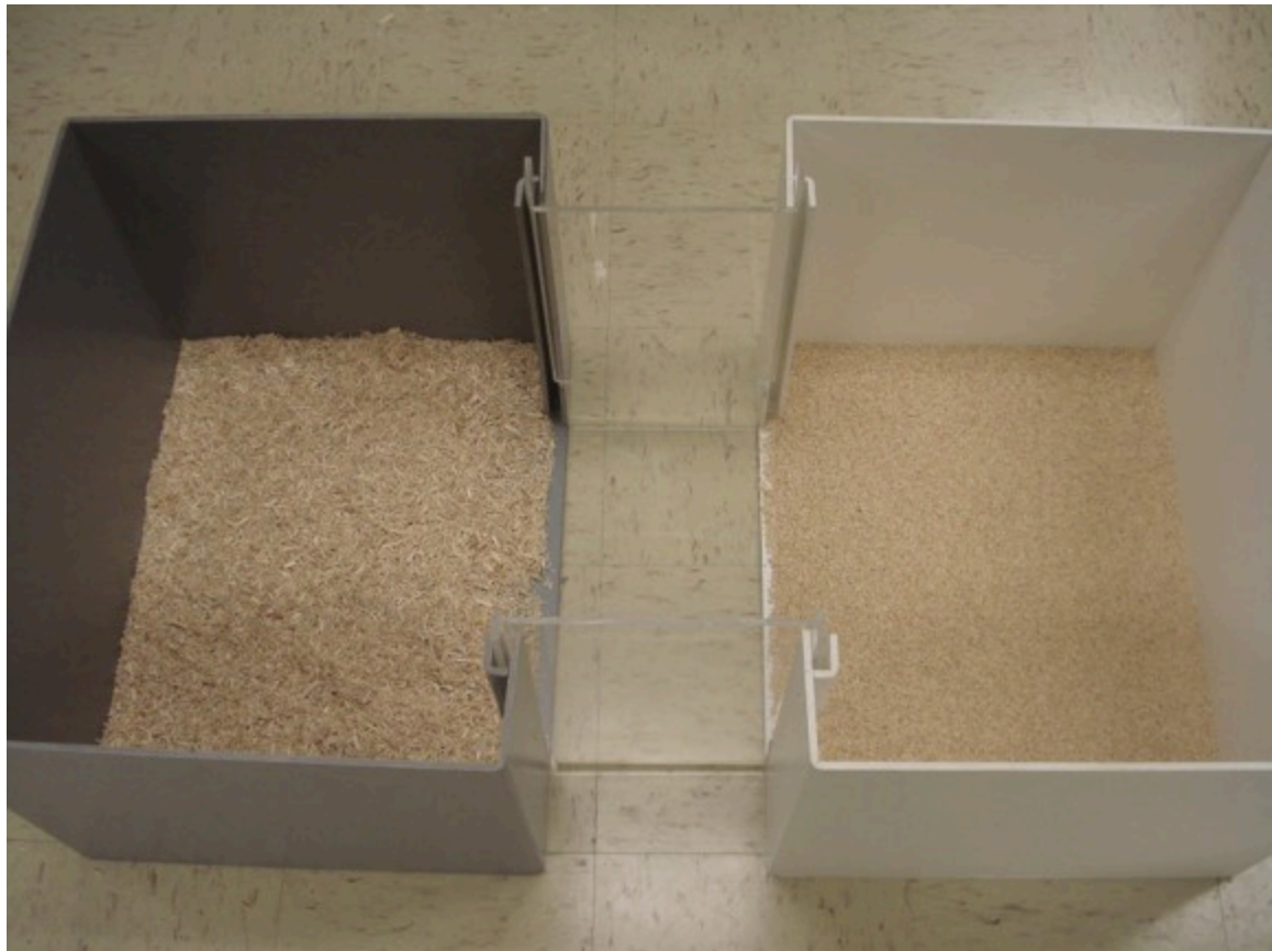
Figure 50.2. Conditioned place preference apparatus. This conditioned place preference apparatus has a clear central compartment that serves as a neutral area. There are two testing chambers that differ in color and tactile sensation on the floor of the chamber. The gray chamber has soft aspen bedding and the white chamber has hard corncob bedding. During testing, a potentially rewarding stimulus is paired with a specific environment (eg. gray chamber) whereas the opposite environment is not paired with any substance or behavior. 'Conditioned place preference apparatus' by Valerie Hedges is licensed under a Creative Commons Attribution-NonCommercial-ShareAlike 4.0 International License.
